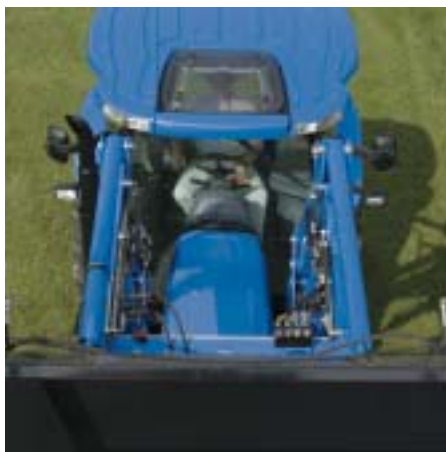
This unique high-visibility panel on the cab roof gives you outstanding visibility to the loader bucket and can be opened for natural circulation.
