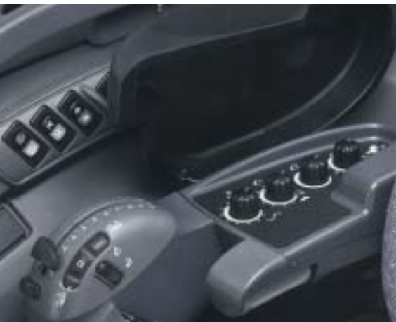
Deluxe cab models include controls for electronic draft control located conveniently on the right-hand armrest console, with additional hydraulic controls under the armrest.
