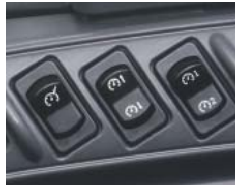
The Constant Engine Speed feature on the TS125A and TS135A allows you to pre-set two engine speeds. Use one for a constant working RPM, then toggle to the lower RPM to turn at the end of the row.
