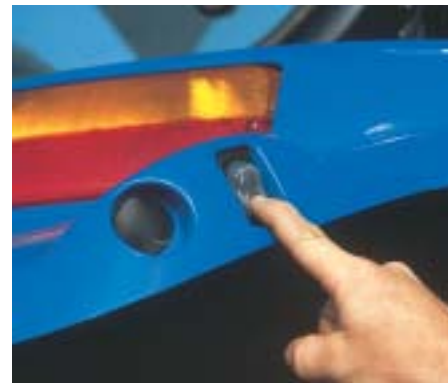
Rocker switches on the rear fenders (on deluxe cab tractors only) allow you to raise and lower the three-point hitch for easy implement attachment.
