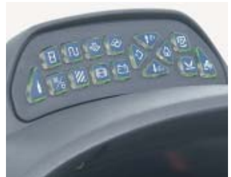
This enhanced performance monitor (on deluxe cab 16 x 16 models), allows you to track and program a variety of functions including linkage height, PTO speed, hours, distance traveled and electronic remote valve status. It also includes a maintenance reminder and an odometer.
