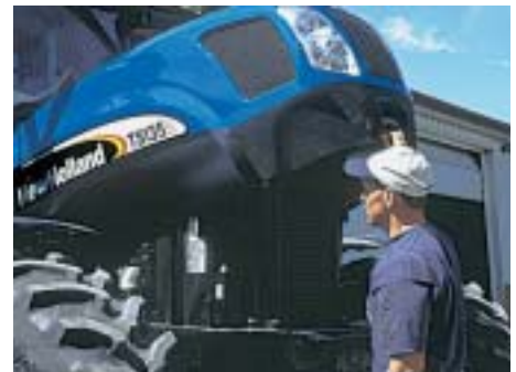
The convenient, one-piece hood opens effortlessly on gas struts to provide access for routine maintenance. The oil cooler and A/C condenser slide out to the side for easy cleaning.
