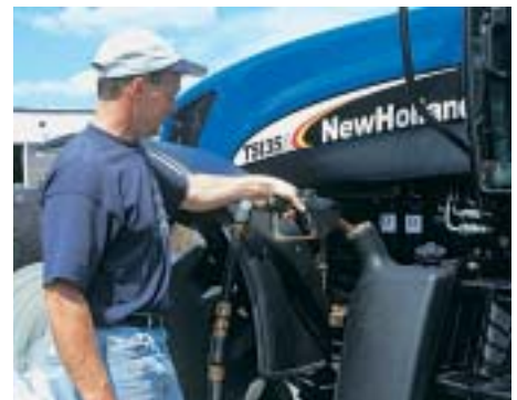
Fueling up from ground level saves time and effort. A 58.1-gallon tank is standard on the largest three models with a 46.7-gallon tank on the TS100A.
